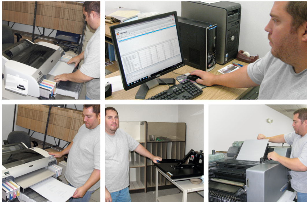
Scharer using the ColorBurst CTP system for print production at CP&G. From top, clockwise: loading the plate in the printer using the plate guide for proper alignment; processing a job to build plates in the ColorBurst CTP RIP; removing the printed plate from the printer; heat-curing the plate in the ColorBurst Plate Press; loading the finished plate in the press.
